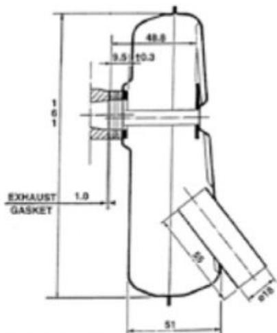
MEASUREMENTS SHOWN HAVE A TOLERANCE FACTOR OF  $\pm 0,3$  mm
